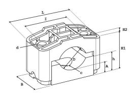
Initial torque for fastening fixing material : 5 - 8 Nm. (depends on cable manufacturer's prescription).
