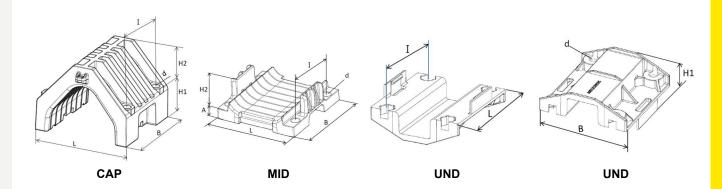
Initial torque for fastening fixing material: 8 Nm. (depends on cable manufacturer's prescription).
