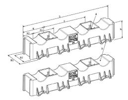
Initial torque for fastening fixing material : 5 - 8 Nm. (depends on cable manufacturer's prescription).
