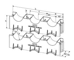
Initial torque for fastening fixing material : 5 - 8 Nm. (depends on cable manufacturer's prescription).
