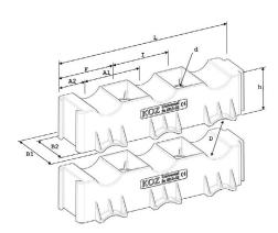
Initial torque for fastening fixing material : 5 – 8 Nm. (depends on cable manufacturer's prescription).
