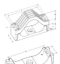
Initial torque for fastening fixing material : 5 - 8 Nm. (depends on cable manufacturer's prescription).
