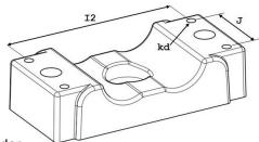
Initial torque for fastening fixing material : 5 - 8 Nm. (depends on cable manufacturer's prescription).
