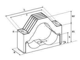
Initial torque for fastening fixing material : 5 - 8 Nm. (depends on cable manufacturer's prescription).
