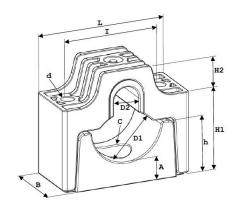
Initial torque for fastening fixing material : 5 - 8 Nm. (depends on cable manufacturer's prescription).
